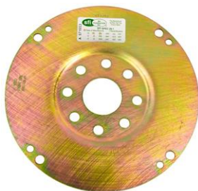
An aftermarket flexplate with both 5/16" and 7/16" torque converter mounting holes can solve a lot of issues.
